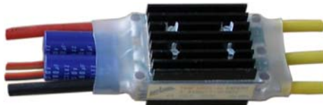
ESC with external short heatsinks (38 mm)
