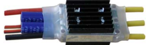
ESC with external heatsinks (38 mm)
