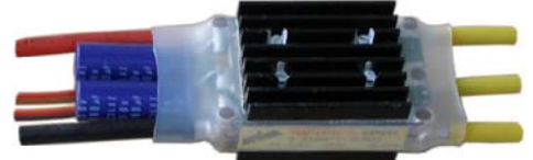
ESC with external heatsinks (38 mm)
